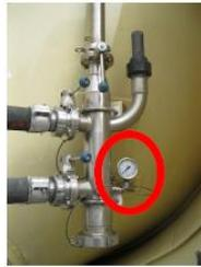
**Step 2:** Start with **building up pressure** by running **compressor** and **opening top air valve**. Also use Aerater from start. Max pressure depending customer.
