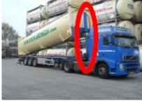
**Step 3:** When **backend is empty** **start tipping** upto **3 cylinders** and unload as normal. To check if empty tip maximum at end of unloading.
