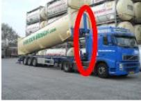
**Step 4:** **When backend is empty**, start **tipping** and unload further with use of top air and injector air. Aerator only when needed.
