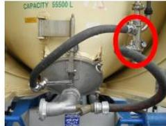
**Step 3:** **Open the injector air** and the **product valve** and start **unloading**. Open product valve max, injector air should be opened (approx half open) until pressure stays around 1 bar.
