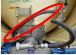
**Step 3:** **Open the aerator to stir up** the product to unload. (not continuously open to prevent product to heat up to much.)
