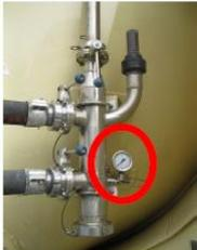
**Step 1:** Start with **building up pressure** by running **compressor** and **opening top air valve**.
