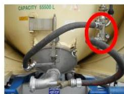
**Step 3:** **Open the injector air** and the **product valve** and start unloading. Injector full open, product valve semi open.
