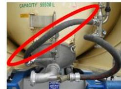
**Step 4:** **Aerator open** during unloading process. Valve approx half open during all unloading.
