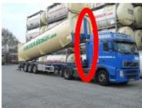
**Step 1:** Start with **tipping max cylinder** (5/6 depending on chassis).
