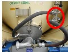
**Step 3:** **Open the injector air** and the **product valve** and start **unloading**. Open product valve max, injector air should be opened (approx half open) until pressure stays around 1 bar.
