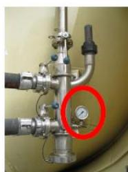
**Step 2:** Start with **building up pressure** by running **compressor** and **opening top air valve**.
