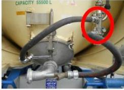
**Step 2:** **Open the injector air** and the **product valve** and start unloading.
