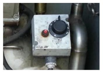
**Single thermostat:** The desired temperature can be set by turning the knob to the specified temperature.
