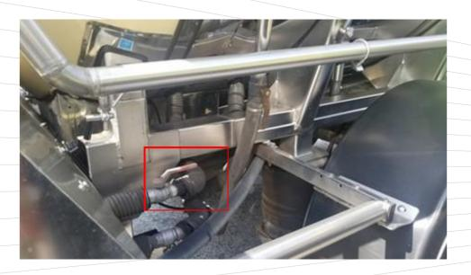
If there is no shut-off value in the heating box, then the position of the value is automatically correct. However, note that it must be in the correct position in front of the tank as well. Also check if the pump is turned on (pump makes noise and vibrates).
