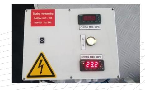
**Chocolate thermostat:** The desired thermostat can be selected by turning the switch in the middle. The top thermostat should be used with chocolate. This thermostat prevents chocolate from burning and cannot be set higher than 55 C°.
