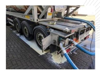
A leak is inconvenient, time-consuming and may be dangerous. It is harmful to the environment and can damage the product. It also damages your reputation. Therefore, always check your equipment. This also takes time, but that does not outweigh all the disadvantages of a leak.
