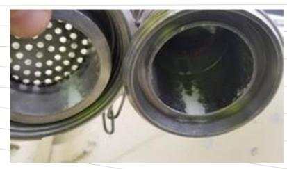
Couplings and unloading elbow are stored in clean state. Also check the functioning and cleanliness of the one-way valve on the unloading elbow.
