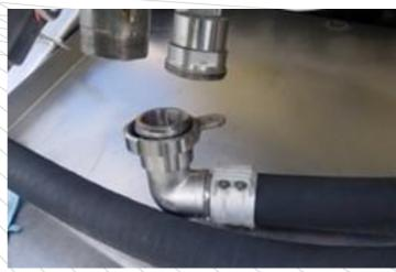
Clean the couplings and coupling chest as well as the couplings and coupling chest of the truck.
