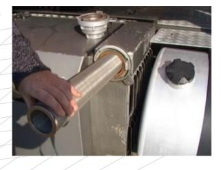
Make sure the dry bulk compressor filter (if present) is clean and placed in the casing. If the filter is not clean, report this to the planner. The filter should then be cleaned. The presence of oil may indicate an internal leak in the compressor.
