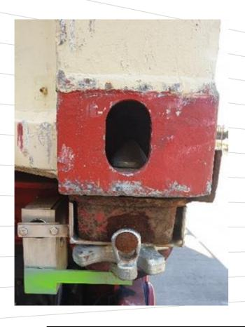
Twist lock with N/O contacts. The twist lock must be closed entirely to prevent the tilting mechanism from being short-circuited. It is impossible to tip if the twist lock is not fully closed and both points do not make good contact. Dirt and water also prevent good contact.
